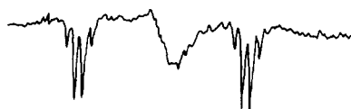
Figure 2. AISEFT spectrum of N -methylacetamide ( ^{15}\text{N} being in natural abundance) with ^{15}\text{N} satellites corresponding to ^1J_{\text{NH}} . Note the smallness of the residual peak corresponding to molecules containing ^{14}\text{N} .
